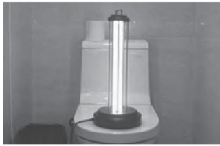
Fig. 6. Disinfection of the toilet with a portable lamp
